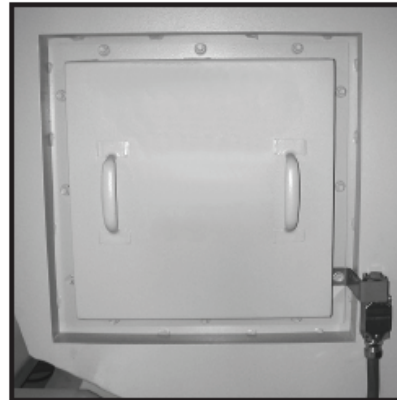
Side cleanout door with safety interlock
